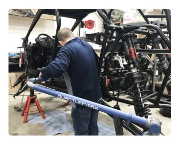
often reverse engineering existing vehicles where CAD data is unavailable to integrate new technologies into fielded platforms," Wilson explained. "Both laser and hard point scanning with the Quantum Max are performed on the actual frame. That includes the chassis and the entire vehicle body on frame."
