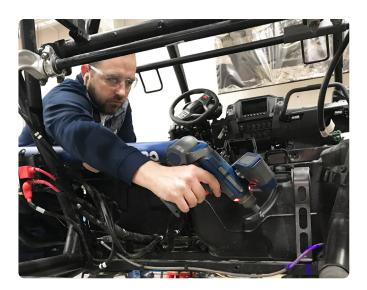
With advantages like these it's clear the Quantum Max, used as a tool to reverse engineer off-the-shelf parts, will continue to be an invaluable tool for the burgeoning electric vehicle market, especially as the industry at large continues to gain traction with middle class consumers and the general driving public.
