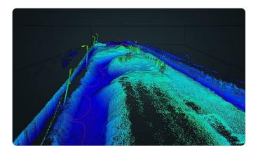
The SLAM solution is ideal for rapid data capture and has the capacity to process in real-time. By walking through the construction and demolition waste sites, the team is mapping as they go, shortening the amount of time spent in a hazardous environment — reducing health and safety risks.
