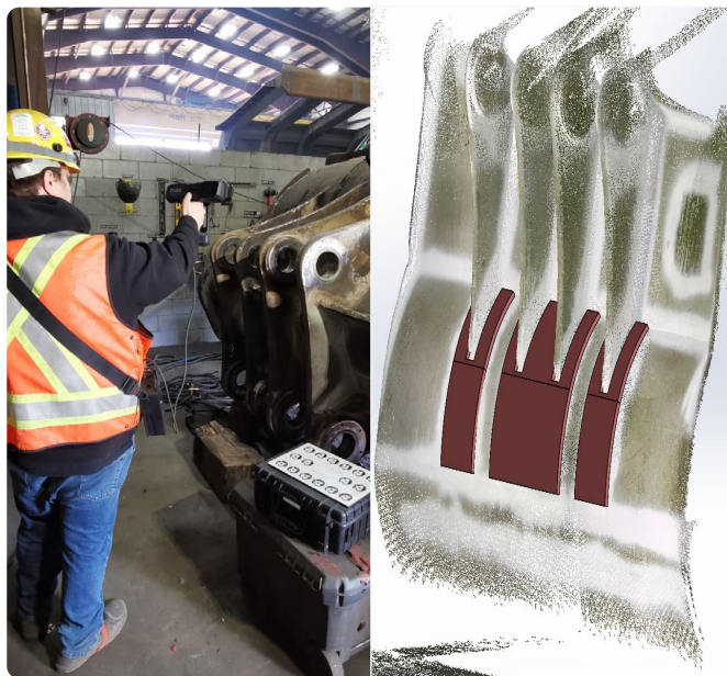
Heavy mining equipment frequently has complex, curved pieces that are challenging to measure by hand. Pictured here is a Hitachi excavator bucket that needs to be refurbished.
