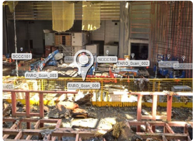
Photorealistic 3D scans obtained with the FARO Focus M 70 Laser Scanner ensures evidence doesn't get missed out, and allows users to virtually 'walk-through' the scene.
