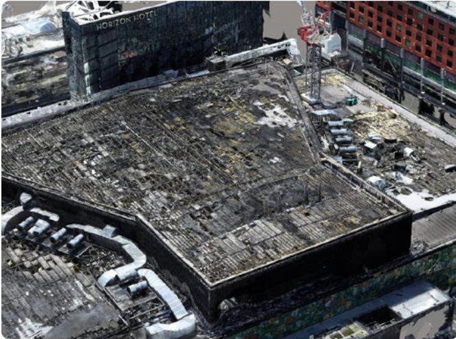
Drones provide context and perspective of the extent of damage in fire investigations, but other tools and methods are required to preserve finer details.
