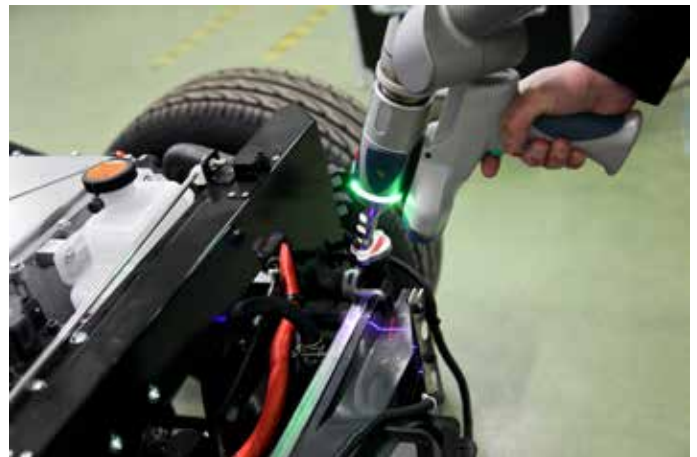
Measuring the EV platform using the FARO Edge ScanArm HD.
