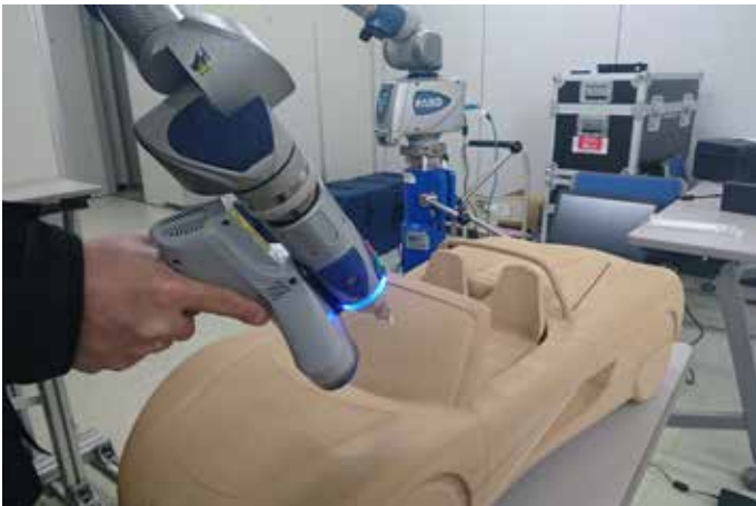
Scanning a mock-up, which will be utilized for the actual EV development.
