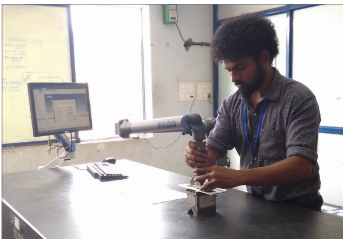
An operator uses the FaroArm's contact probe to inspect a sheet metal product for accuracy.
