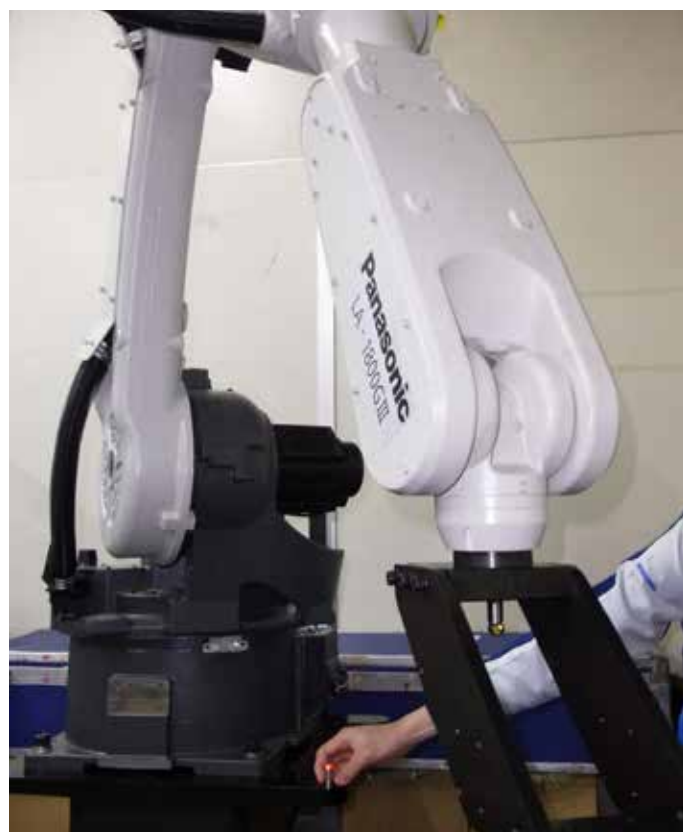
Measurement of the pedestal of a medium-sized versatile robot manipulator LA-1800. Arm gauge SMR (retro reflector) for measuring marks is also attached.
