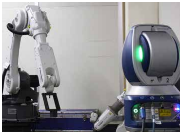
FARO Vantage and BuildIT Metrology Software accurately measure the trajectory of the robot arm.
