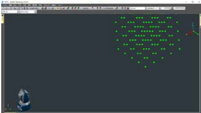
Trajectory of robot arm displayed on BuildIT Metrology software. It can be obtained not by relative position but by absolute position.
