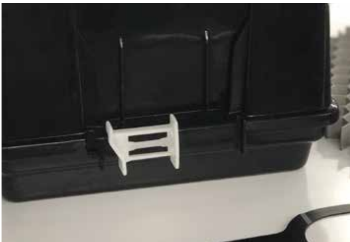
A discontinued part can be easily replaced through the reverse engineering process — scan, model, and 3D print.
