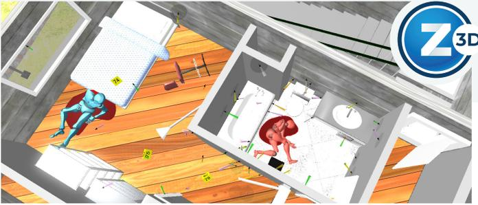
For forensic investigators, FARO Zone 3D provides the ability to accurately reconstruct any crash, crime, or fire scene. Apply manual measurements, aerial maps, drone photos, or total station data to quickly create 2D and 3D scene diagrams. Analyze the scene with crash reconstruction, bullet trajectory, and blood spatter analysis tools. Create compelling walk-throughs, reports, and animations to present the case.
