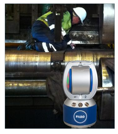
over to one side. Another trend is a developing misalignment between parts like motors, gears, bearings, and rolls. Because we can capture measurements from multiple parts at once with the Vantage, we can determine if there's misalignment between parts, wear of a particular part, or if the whole darn thing is leaning over."
