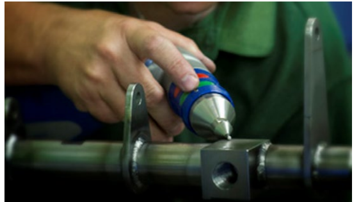
Inspection using FARO Gage
