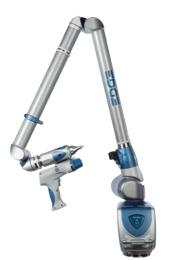
Effort Foundry began its technology transformation by searching for an ideal tool for fast point-cloud collection with high-definition data, repeatable accuracy, and the ability to scan dark and reflective surfaces without spray or targets. After evaluating numerous options, they selected the FARO® Edge ScanArm® HD – a contact/noncontact portable 3D measurement system that combines all of the advantages of tactile measurement with a 3D scanning attachment utilizing blue-laser technology.
