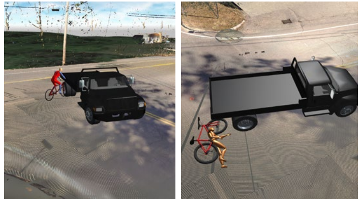
These images are frames in the animation Lakowicz created using FARO Zone 3D. The left image shows the point of impact and the right shows the final rest position of the bicycle, as determined by the measurement data and the photogrammetry analysis of the scene.
