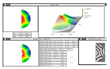
Figure 8: Interferogram Demonstrating Wavefront Distortion
