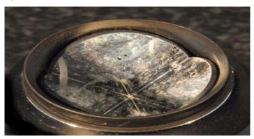
Gold coatings are primary reflective surfaces and are not susceptible to oxidation as is silver. The gold color is also more reflective to some ADM wavelengths and will enable longer range performance. Gold surfaces are more susceptible to scratches during cleaning but comprehensive tests have shown that these micro scratches do not impact SMR performance.
