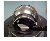
nine measurements. The SMR should be in the starting position at the end of the test. In any measurement application, best fit a point with the nine points and review the form. Due to the various SMR specifications and tracker accuracies it is not possible to provide a tolerance range for the form error. The tracker vendor should be able to provide an expected error or the operator can test a new SMR in a good environment and use this as a baseline for future runout checks.
