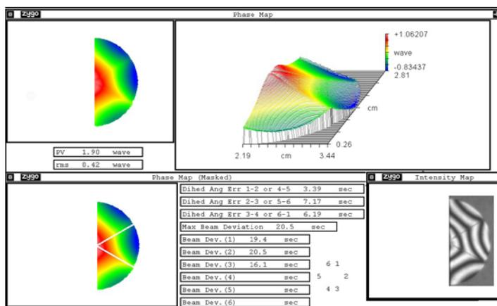
**Figure 8:** Interferogram Demonstrating Wavefront Distortion
