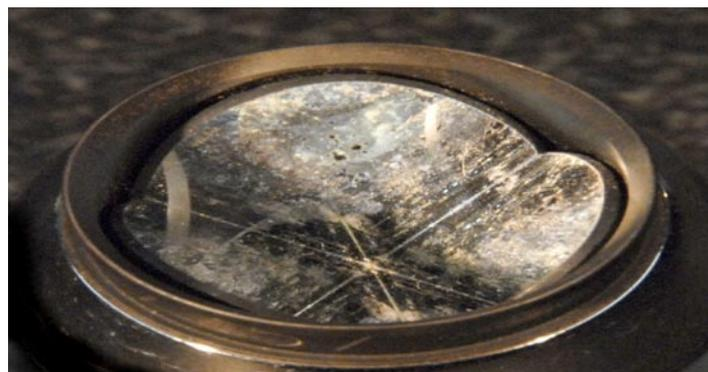
Gold coatings are primary reflective surfaces and are not susceptible to oxidation as is silver. The gold color is also more reflective to some ADM wavelengths and will enable longer range performance. Gold surfaces are more susceptible to scratches during cleaning but comprehensive tests have shown that these micro scratches do not impact SMR performance.
