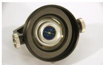
are not centered properly and the beam will not return round, but oblong. Other aberrations in the beam can be caused by a non-uniform bond layer or areas of the glass surface that are not spherical. Generally, cateyes are constructed very well and the operator only needs to be concerned about not clipping the beam in an effort to maximize the acceptance angle of the target. It is possible to still track while beginning to clip the beam so care must be taken in the use of a cateye target.
