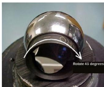
**Depth Error:** Place the SMR in the nest as in the runout test. In this test we want to rotate the SMR in a horizontal plane about 20 degrees to the left and take a point and then to the right about 20 degrees
