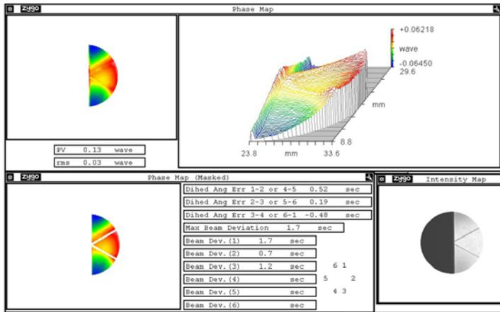
**Figure 7:** Interferogram Demonstrating Dihedral Angle Error
