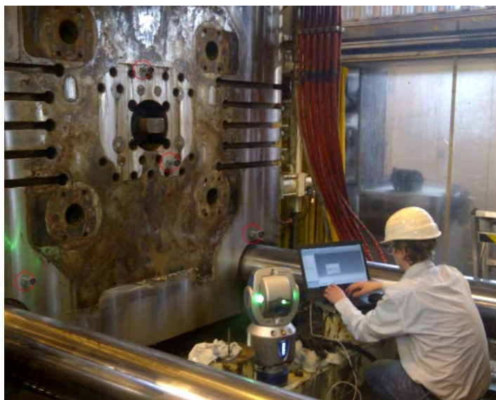
Observation from different reflectors on the room, to recognize move or drift on-load.
