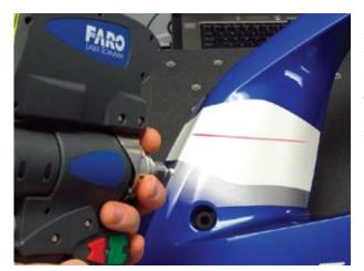
Synergeering can laser scan customers' parts and create fully-surfaced 3-D CAD models, then produce fully functional components from their unique rapid prototype capabilities, and deliver within days.
