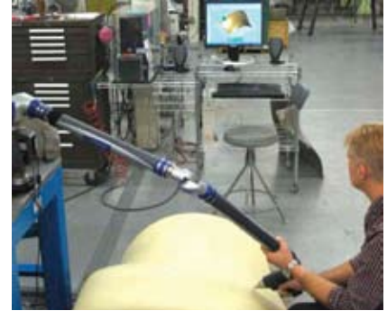
Reverse engineering the original Master Molds into CAD
