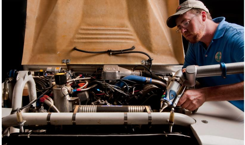
Additionally, the Jackson Jonson team utilizes the Edge to measure bent stainless steel tubes that are used in the Air Force One Performance Industries' automotive cold-air intake kits. The Edge has allowed them to quickly find the centerline bend radii on the tubes, as well as quickly model the assemblies with accurate hole placements, weld-on attachment placements, etc.
