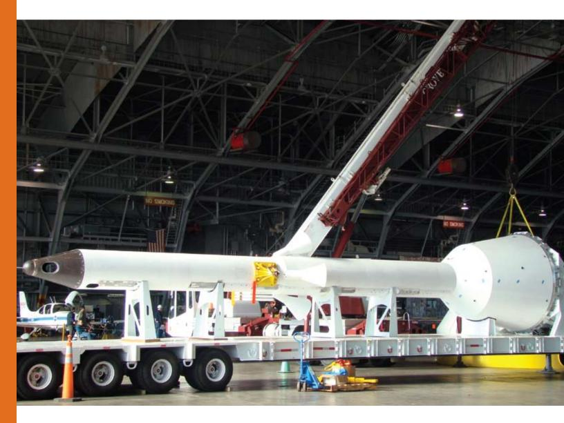
NASA Langley Research Center is facilitating the build-up of the Ares I Crew Module, the Launch Abort System and the Separation Ring Assembly. With the high accuracy requirements when building these items, the Research Center has turned to laser tracker technology. Laser trackers are recognized in the aerospace industry for their portability, ease-of-use and their ability to achieve extremely high accuracy levels.
