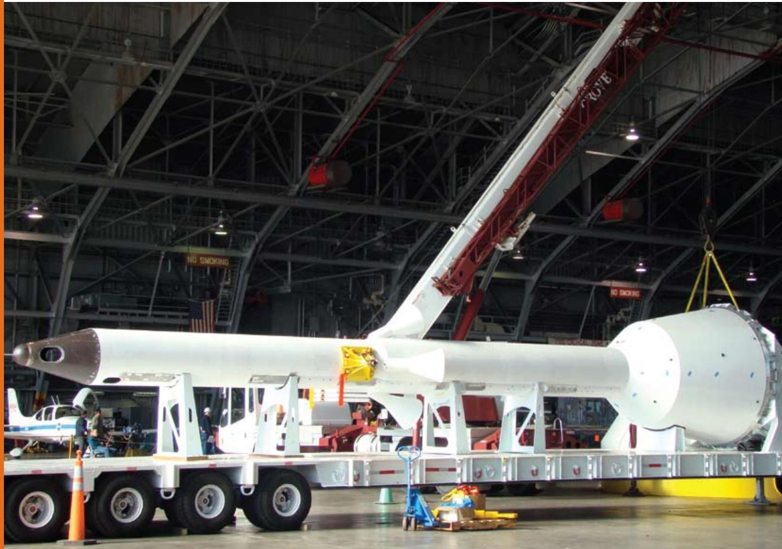
NASA Langley Research Center is facilitating the build-up of the Ares I Crew Module, the Launch Abort System and the Separation Ring Assembly. With the high accuracy requirements when building these items, the Research Center has turned to laser tracker technology. Laser trackers are recognized in the aerospace industry for their portability, ease-of-use and their ability to achieve extremely high accuracy levels.
