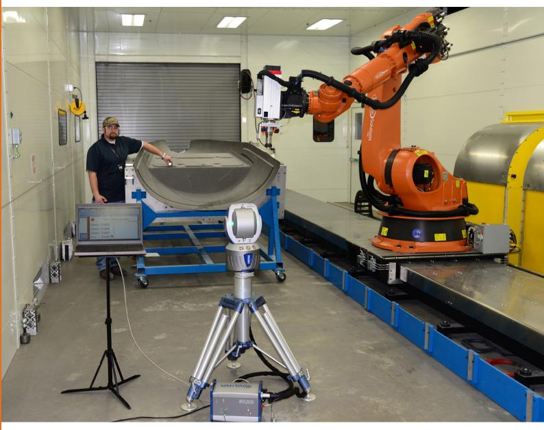
"Though the robot calibration is a unique application, Cirrus has also utilized the Tracker with other large scale needs such as assembly and bond fixture setup, component inspections, and even entire aircraft inspections. The FARO Laser Tracker has and will continue to be a valuable tool in Cirrus Aircraft's arsenal of success, both now and into the future."
