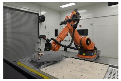
30.9 feet long. Smaller parts, parts as small as 6-inches x 4-inches x 2-inches, can also be cut by the robot while being held in place by a vacuum table. Larger parts, however, utilize dedicated holding fixtures.
