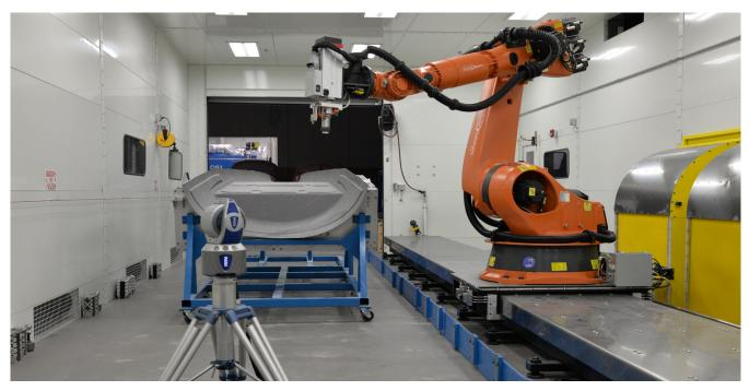
degrade the overall accuracy below the acceptable limits after several iterations. Being able to measure any point in the robot cell with the Tracker has proven to be critical to the process.
