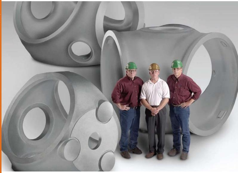
Previously, ATI Casting Service used a combination of a fixed CMM, a laser calibration system, and an interferometer to measure their wind turbine hubs, which are often approximately eight feet in diameter. This assortment of devices was complicated to use, was not very fast, and did not offer the reporting that is so often required today.
