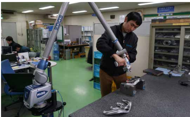
The FARO Edge ScanArm is a portable CMM that is shaped like a human arm
