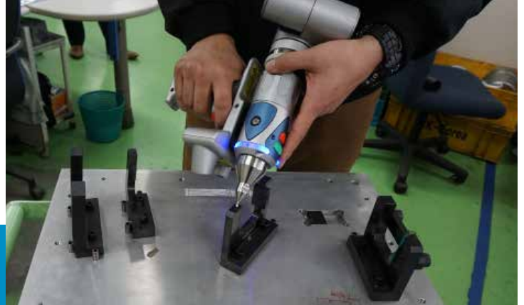
Calibrating an inspection fixture with a tactile probe.
