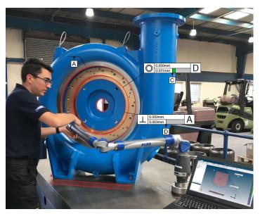
The ability to run FARO CAM2 from a portable laptop ensure maximum portability and flexibility.
