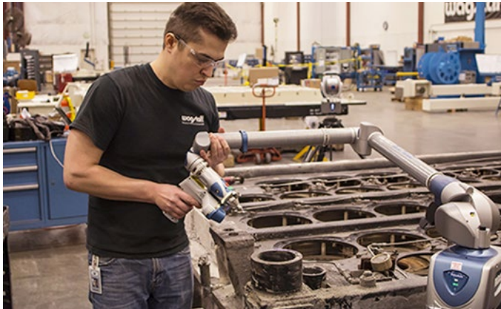
Aleksandr Bakhtin scanning mating components to determine if there are any alignment issues.
