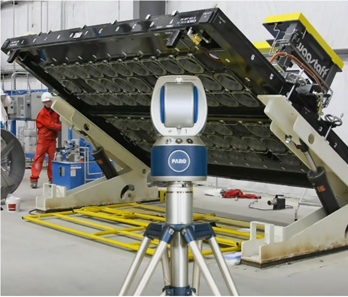
Each mold table is mated to a custom Wagstaff Mold Table Mounting System.
