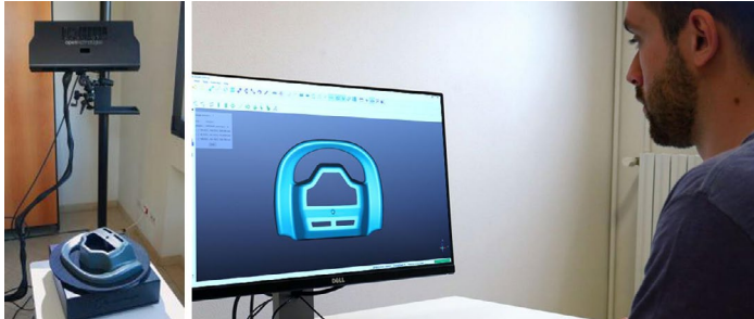
A structured light 3D scanner projects patterned white light onto an object. (Images courtesy of Open Technologies.)
