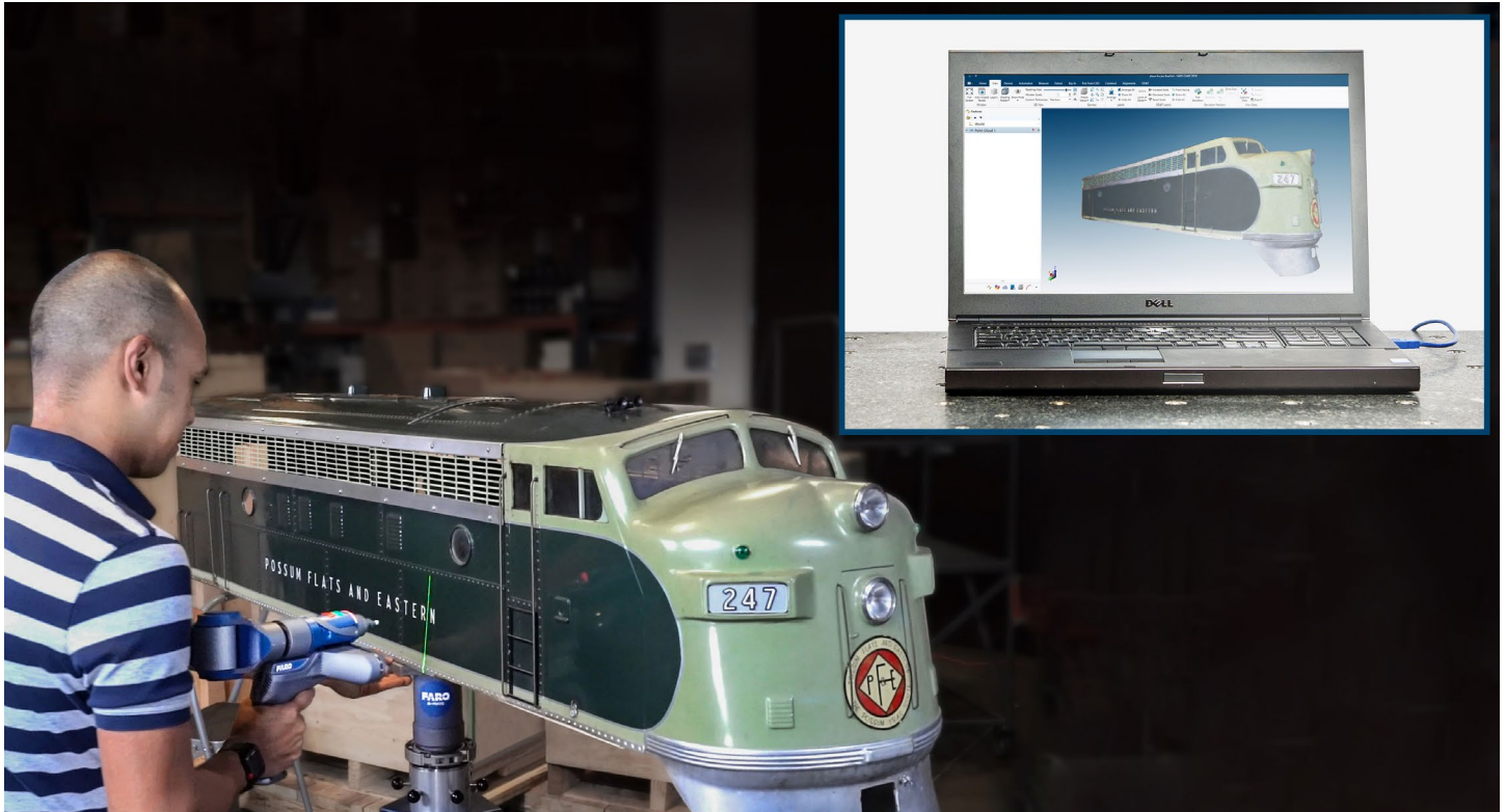
A large model train sits atop the rotary stage to make scanning the complete object much easier for the user. (Image courtesy of FARO.)
