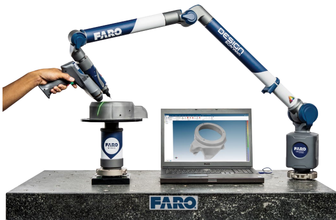
The eighth axis of the FARO 8-Axis Design ScanArm is the rotary stage in the center. (Image courtesy of FARO.)
