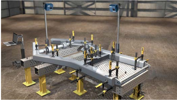
Figure 3. Two Tracer M projectors at work in an assembly operation.
