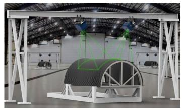
Figure 2. Two Tracer<sup>M</sup> projectors projecting onto an engine nacelle for ply layup in a composites clean room
