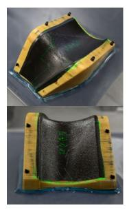
Figure 4. Projection onto a composite winglet mold.
