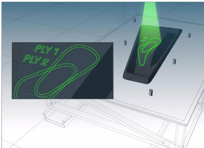
Figure 3. Tracer<sup>M</sup> projection of multiple plies onto a composites mold
