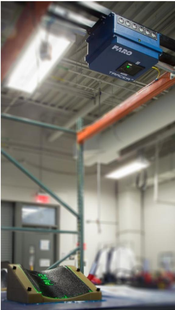
Figure 1. A Tracer<sup>M</sup> projecting onto a winglet mold for laser-guided layup in a composites assembly facility.
