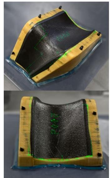
Figure 4. Projection onto a composite winglet mold.
