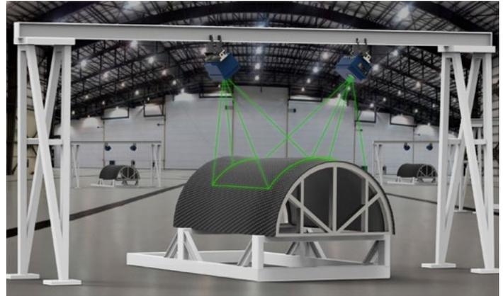
Figure 2. Two Tracer<sup>M</sup> projectors projecting onto an engine nacelle for ply layup in a composites clean room
