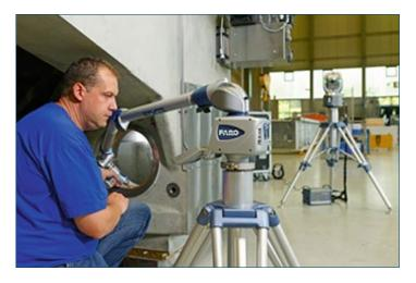
Once that is established we can tie into the tracker's reference system through Polyworks' device localization feature. So now, instead of locking into tooling points, you connect the FaroArm (which, for the TrackArm solution, has SMRs attached directly to the FaroArm) to the laser tracker and take a couple of thousand points to localize the arm to the tracker. Once that is established, you start scanning the tool with the integrated laser scanner on the FaroArm."
