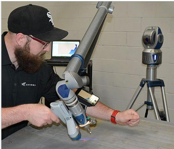
Even with the FaroArm's 12-ft-diameter reach (for the largest model), on a large tool it may be necessary to move the arm from station to station (leap-frog). However, with the Super 6DoF TrackArm solution, because the arm is referenced to the tracker, in the end all of the data sets are already prealigned to the same coordinate system and can all be fit together. Individual fitting is not necessary.
