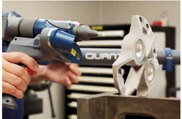
Performing inspection with a FARO Quantum S ScanArm
