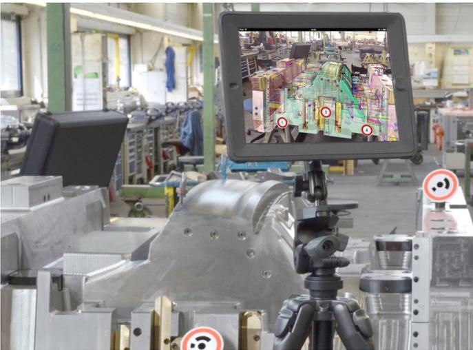
FARO® Visual Inspect™ AR Software enables the intuitive viewing of complex 3D data for (virtual) quality checks of parts and assemblies – even in early stages of an assembly process. Users can, for example, quickly check if all necessary drill holes are in place, and if components (that may not be physically present) will fit in the current assembly.
