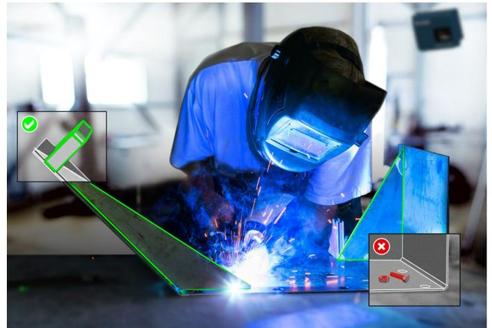
Innovative laser imaging and projection solutions such as the FARO® Tracer<sup>SL</sup> Laser Projector help welders increase throughput by accurately guiding the placement of each part. The solution also allows users to perform IPV, making it perfectly suited for applications such as assembly, alignment, and composites ply-layup, where mistakes, rework and scrap can be extremely costly.
