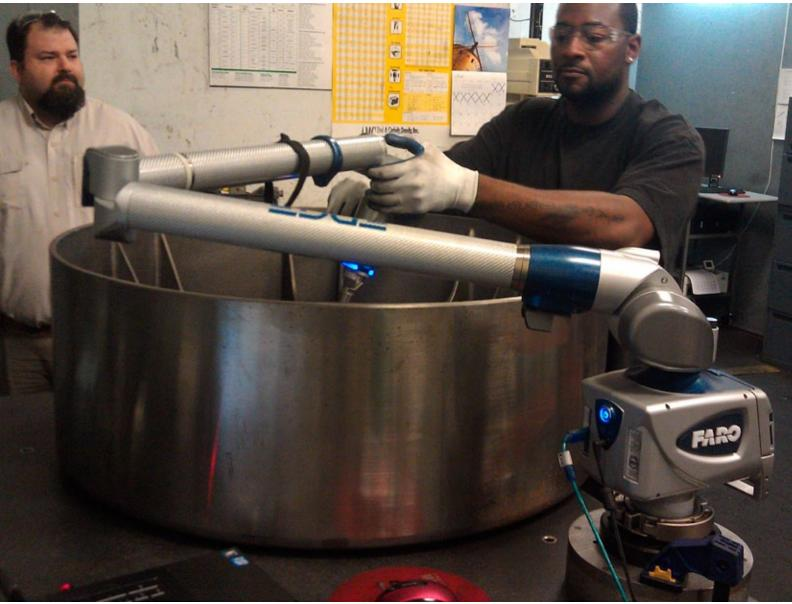
The fast, and easy, setups with the Edge have greatly impacted the overall efficiency of the floor. Total check time for parts that once took 45 minutes and three position changes on a traditional CMM, are now done in only 2 and half minutes using the FARO Edge – a reduction of over 90%.
