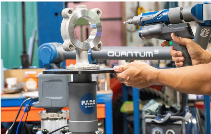
The FARO 8-Axis system delivers innovative real-time part rotation to streamline quality inspection processes
