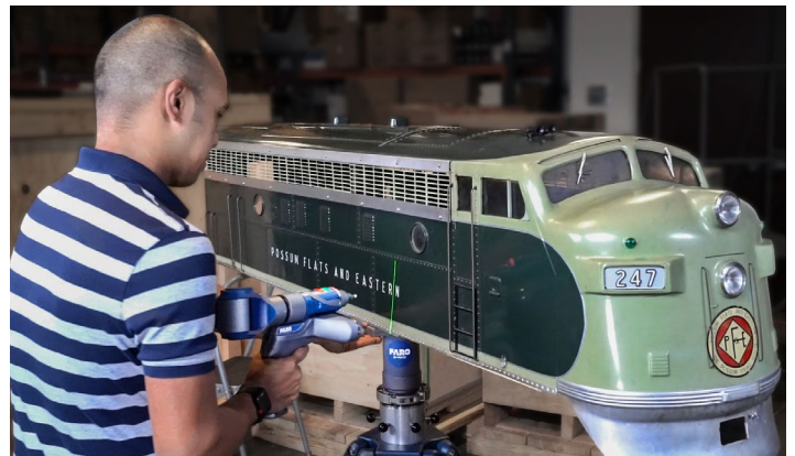
Scanning large objects in color is fast and simple with the 8-Axis ScanArm and PRIZM Color Laser Line Probe
