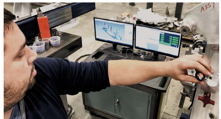
Chad Fortune of Datum Metrology using a BuildIT software and a Vantage E Laser Tracker to measure jig and tooling fixtures at a client's site.
