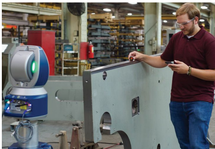
Figure 2. Measuring the Crown of a Press Brake Ram
