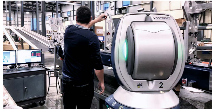
Chad Fortune of Datum Metrology using a Vantage E Laser Tracker to measure jig and tooling fixtures at a client’s site.
