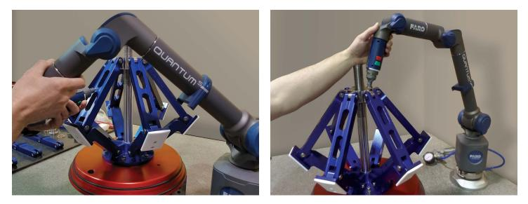
Using a 1.5 meter Quantum<sup>s</sup> FaroArm<sup>®</sup>, the most accurate portable measurement arm on the market, to inspect a precision tool that Woodland Trade built for an aerospace company.
