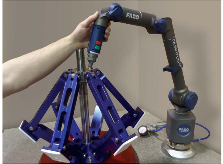
*Using a 1.5 meter Quantum<sup>S</sup> FaroArm®, the most accurate portable measurement arm on the market, to inspect a precision tool that Woodland Trade built for an aerospace company.*
