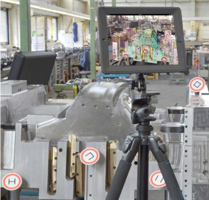
With the tablet's integrated camera, an overlay of the as-built object with virtual 3D data, including all process and workflow information, can be realized in real time.
