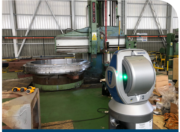
Figure 3. Vantage Laser Tracker performing measurements on a bearing casing
