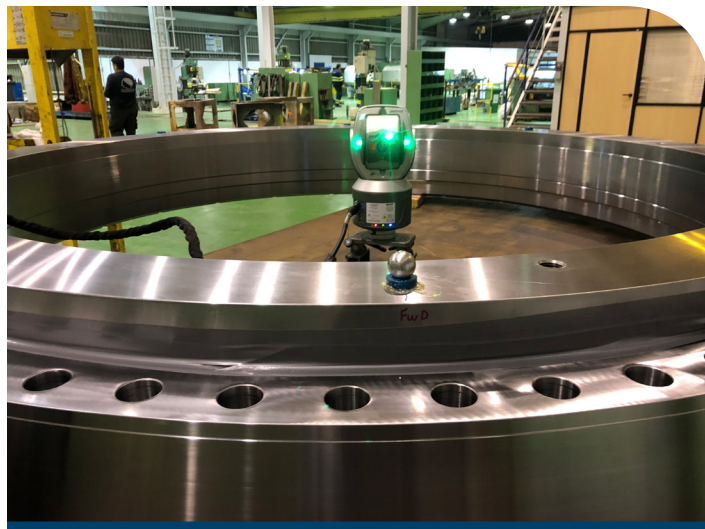
Figure 2. Vantage Laser Tracker doing on-machine measurement during the machining process for a bearing casing
