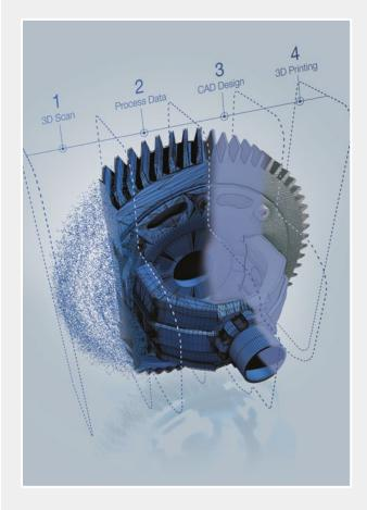
Subsequent software solutions can then leverage the data to create simple or even parametric, native CAD models for quick and accurate changes downstream and to confirm your model to the original scan data to verify design intent. The data can then be aligned, cleaned, meshed and smoothed in preparation for Reverse Engineering.
