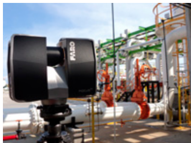
Fig. 3: Capture complex piping structures with a laser scanner
