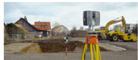
Fig. 7: Volume calculation using a laser scanner
