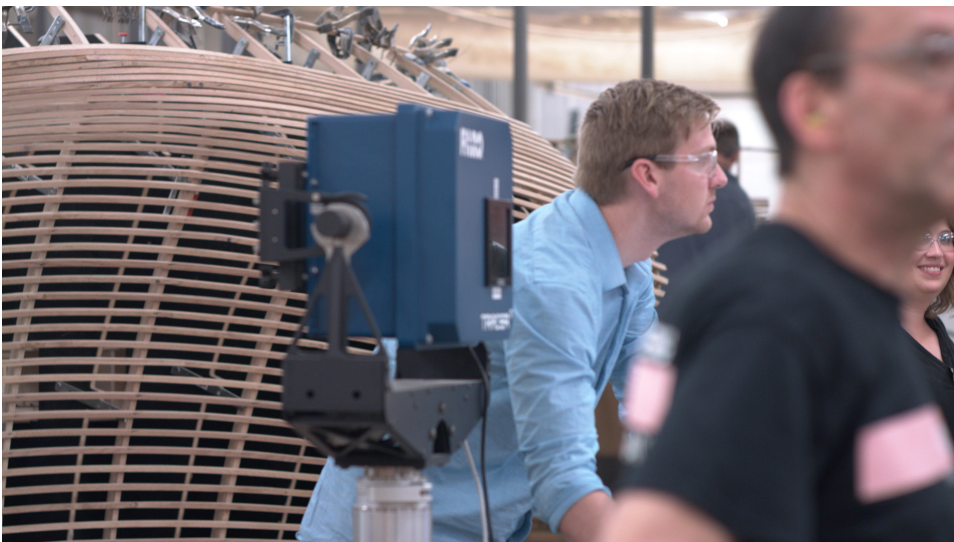
CWKA used the FARO Tracer Laser Projector to assist with panel fabrication. The Tracer projected a template, shown here in green, to guide steam bending and thread placement.
