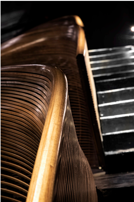
The Tracer allowed CWKA fabricators to place each white oak thread with digital precision, creating swooping and swirling panels.
