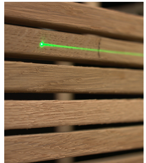
CWKA used the FARO Tracer Laser Projector to assist with panel fabrication. The Tracer projected a template, shown here in green, to guide steam bending and thread placement.
