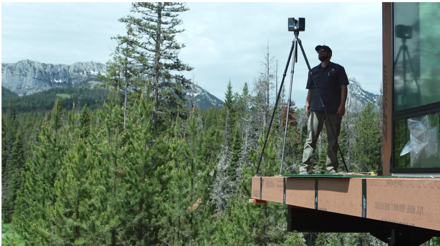
Brandner Design deployed the FARO Focus Laser Scanner to ensure accuracy on a high-end project in Bozeman, Montana.
