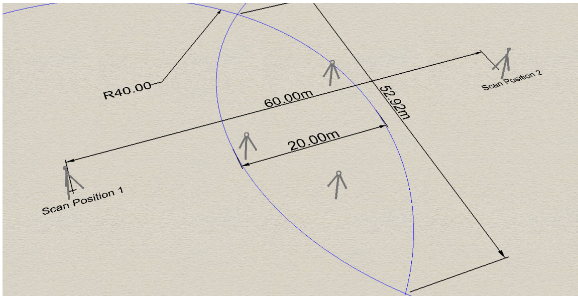
Figure 3. Scanner Test Preplanning Layout: Note: All dimensions in meters
