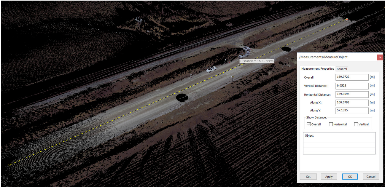
Figure 6. Screen capture from FARO Scene showing a 3D view of the scans.
