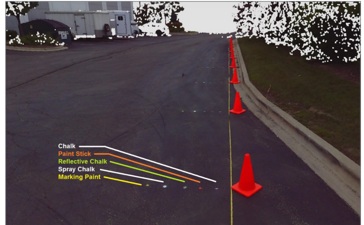
Figure 3. Colorized scan image of the point cloud showing dots.
